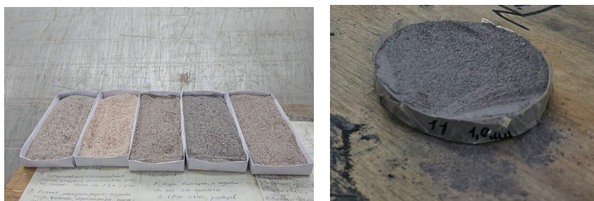
Figure 6 - Crushed Fraction (Left) and Analytical Powder (Right) for XRT
